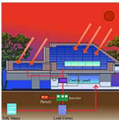
The solar cells generate 22 kilowatt-hours, and can store energy for three days. Surplus energy can be sold to the power company or used to drive an electric car. Image: Chulalongkorn University
